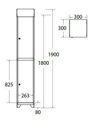
Model WA01 is our floor standing locker. Manufactured from grade 304 stainless steel, this locker has an internal shelf with two lockable doors.
